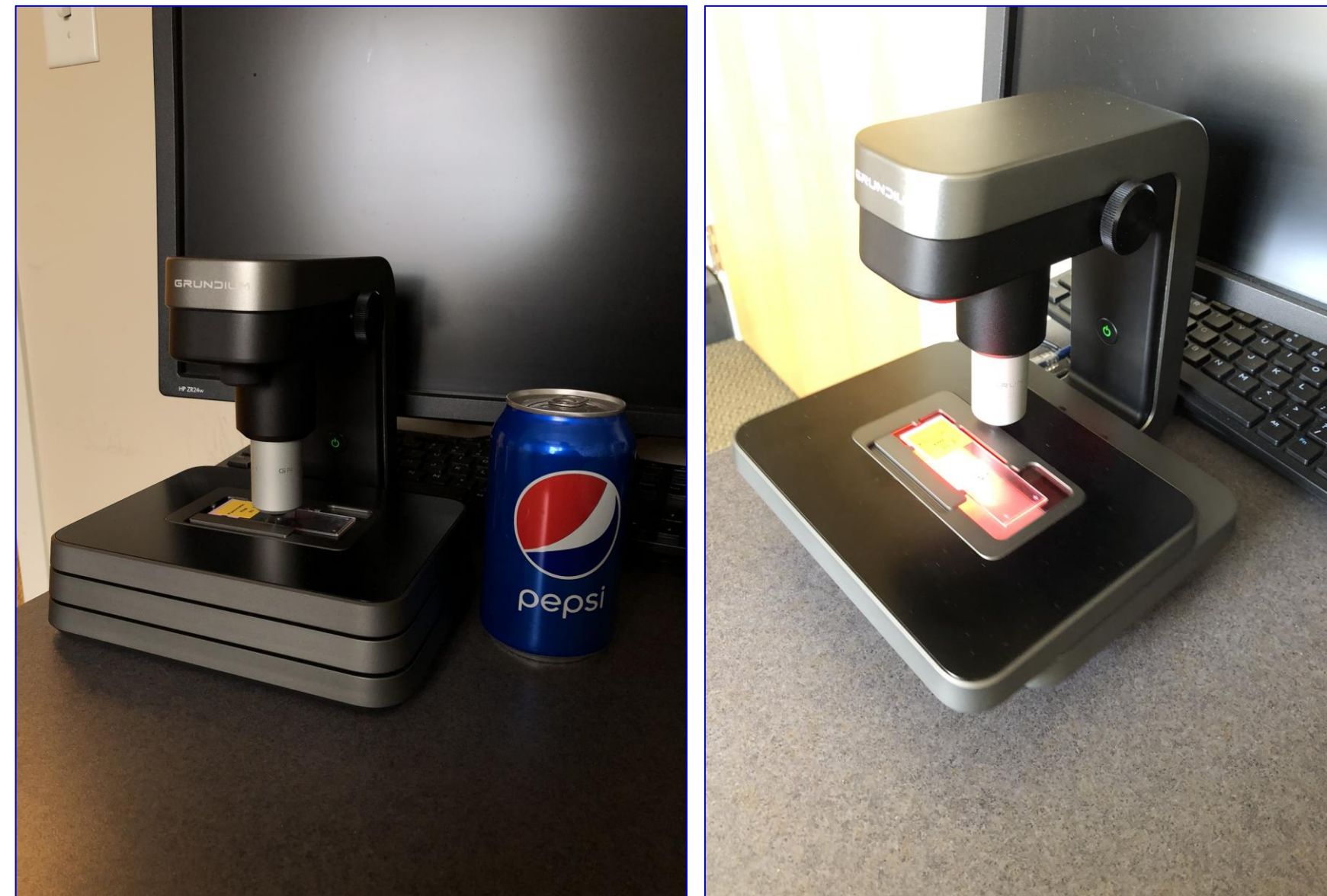
Figure 1. Grundium Ocus® microscope scanner. This desktop hybrid device with 1 slide capacity has a small (3.5 kg, 18 x 18 x 19 cm) footprint.
